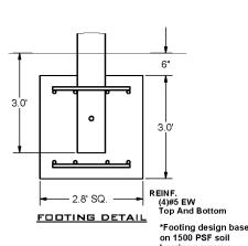
\*Footing design based on 1500 PSF soil bearing pressure.
